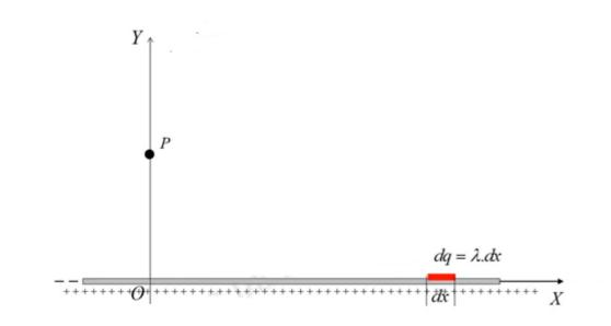
Here we take the rectilinear segment dx that has a charge  $dq = \lambda dx$
