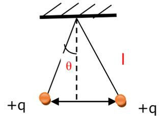
Given:  $\tan \theta \approx \sin \theta$ ,  $m = 10 \text{ g}$ ,  $l = 120 \text{ cm}$ ,  $q = 2.4 \cdot 10^{-8} \text{ C}$ ,  $K = 9 \cdot 10^9 \text{ Nm}^2\text{C}^{-2}$  and  $g = 10 \text{ m/s}^2$ .
