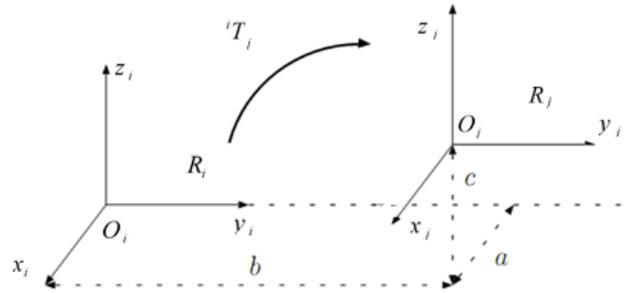
$${}^i T_j = \begin{bmatrix} s_x n_x a_x p_x \\ s_y n_y a_y p_y \\ s_z n_z a_z p_z \\ 0 & 0 & 0 & 1 \end{bmatrix} = \begin{bmatrix} {}^i R_j & {}^i P_{O_j} \\ 0 & 0 & 0 & 1 \end{bmatrix}$$
