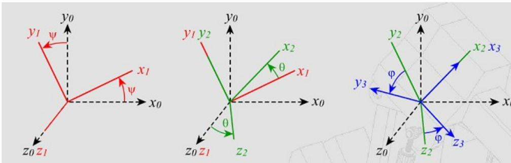
$${}^0R_3 = \begin{bmatrix} \cos \psi & -\sin \psi & 0 \\ \sin \psi & \cos \psi & 0 \\ 0 & 0 & 1 \end{bmatrix} * \begin{bmatrix} \cos \theta & 0 & \sin \theta \\ 0 & 1 & 0 \\ -\sin \theta & 0 & \cos \theta \end{bmatrix} * \begin{bmatrix} 1 & 0 & 0 \\ 0 & \cos \phi & -\sin \phi \\ 0 & \sin \phi & \cos \phi \end{bmatrix}$$
